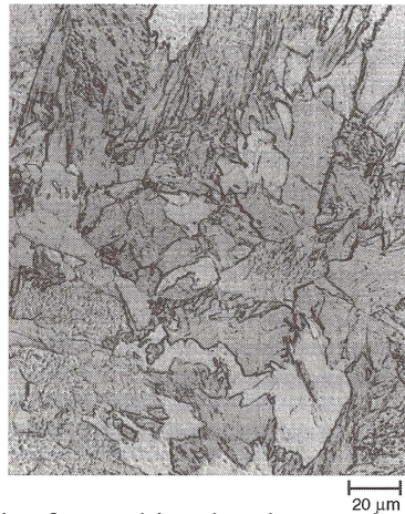
Figure 2.11: Massive ferrite formed in ultra low carbon steel containing 0.003% C and 3.00% Mn cooled at 50°C/s (Krauss 2005).
