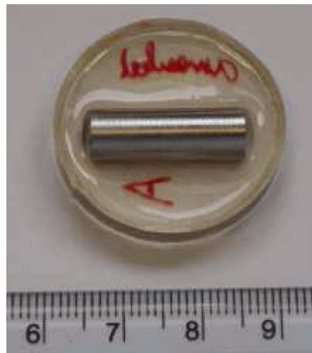
Figure 3- 9: Fixing of microhardness specimens.
