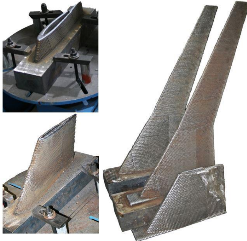
Figure 1:1. Entire demonstrator winglets built by Wire-Arc Additive Manufacture (WAAM), adapted from [2].
