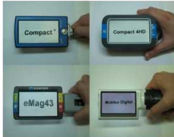
Figure 1. The four p-EVES devices selected for use in the p-EVES study: Optelec Compact+ (upper left), Optelec Compact 4HD (upper right), Schweizer eMag43 (lower left), Eschenbach Mobilar Digital (lower right).
