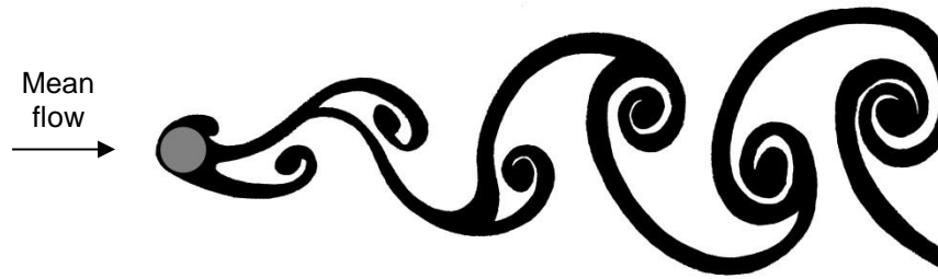
Figure 3.3 - Schematic sketch of vortex shedding from a circular cylinder.
