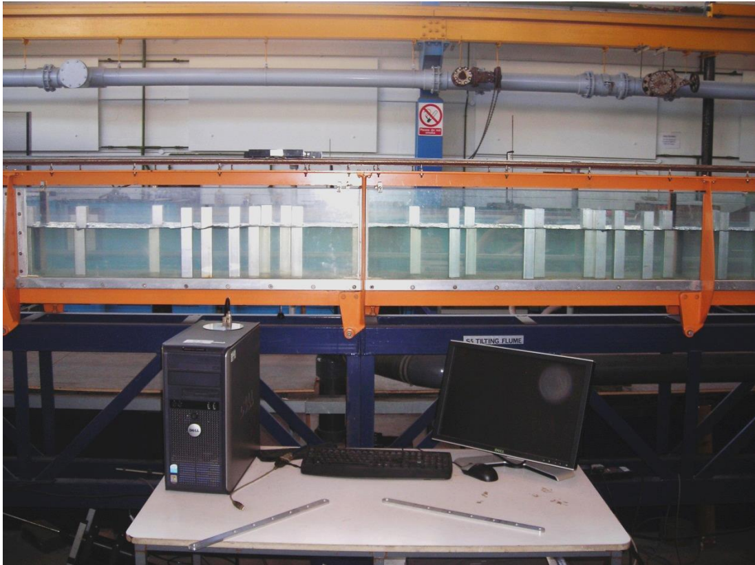
Figure 7.5 - Photograph of uniform flow through random array 2 (3.93% solid volume). The middle section of the flume is shown. Flow enters from the right of the photograph.
