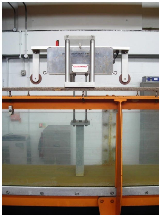
Figure 4.7 - Photograph of the Cussons Single Component Force Balance.
