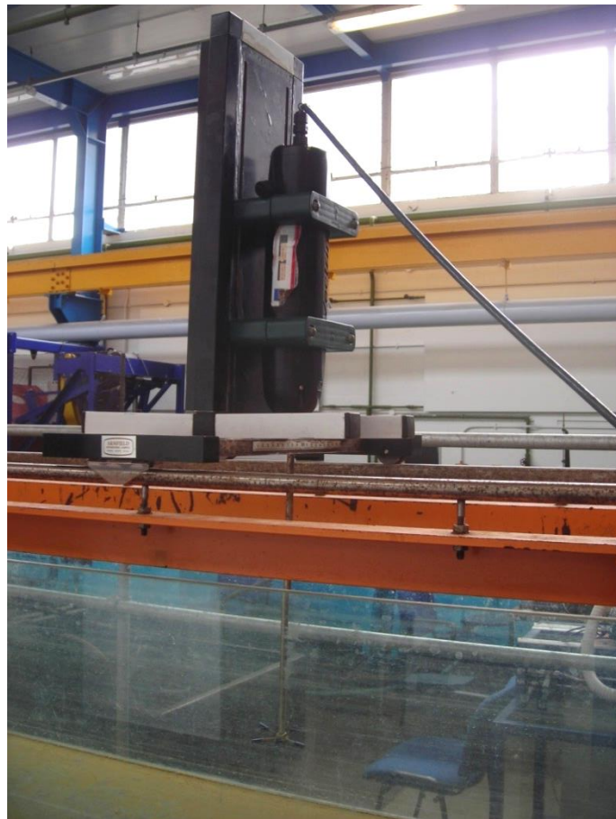
Figure 4.13 - Photograph of the Nortek AS Vectrino Acoustic Doppler Velocimeter.
