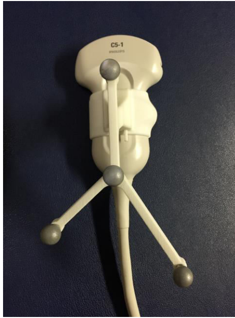
Figure 14: modified US probe with tracking spheres
