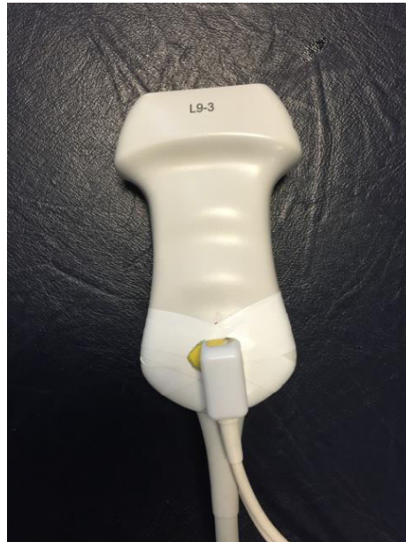
Figure 10: Liner US transducer adapted for magnetically tracked freehand 3D-US. An electromagnetic sensor is attached in a calibrated position.
