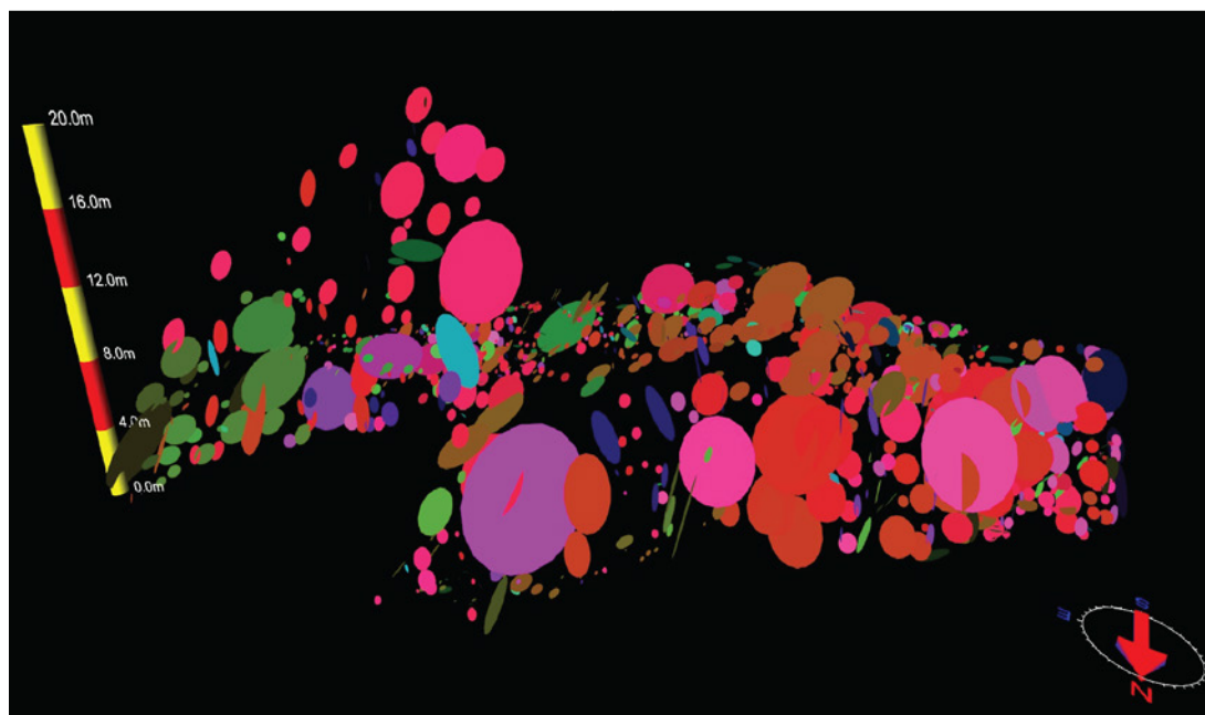
Figure 4.8: Interpreted lidar scan of Rydal Cave. a) shows the raw point cloud data and b) shows the picked fractures. Scale bars are 20 m. Each “disk” shown in the image represents and interpreted fracture, picked by the user. The associated geostatistics can then visualised on a stereonet within the program or be exported and analysed in separate programs. The disk size is not representative of the fracture size, and the colours are arbitrary.
