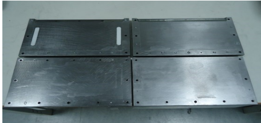
Figure 3-2: Unsuccessful attempt; showing sample stuck to the mould plate.
