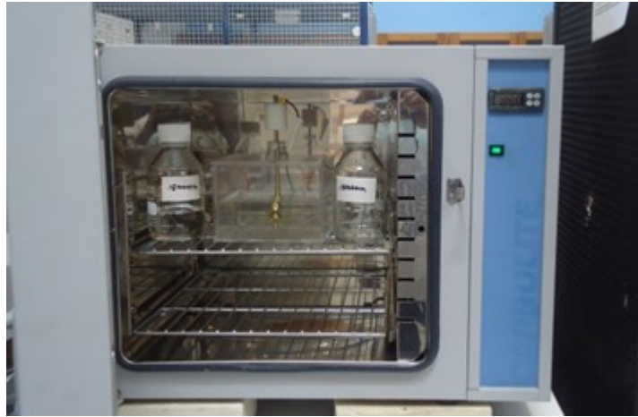
Figure 4-6: Oven where samples and test cell containing oil bath are kept at room temperature prior to testing after conditioning.
