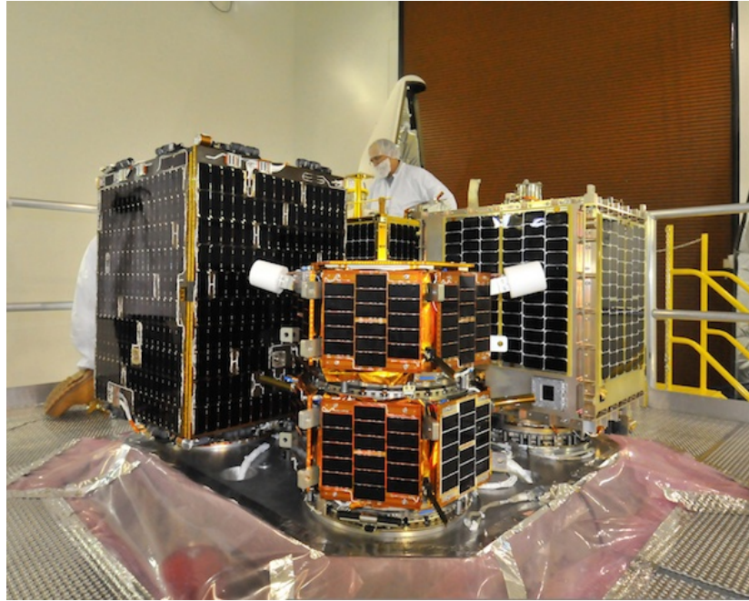
Figure A.1: STP-S26 mission: multiple payloads integrated for Minotaur IV launch [228].
