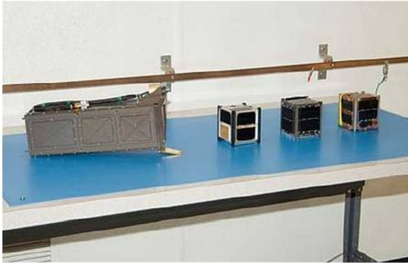
Figure 2.1: P-POD with CP6, HawkSat-1, and AeroCube 3 CubeSats [22].
