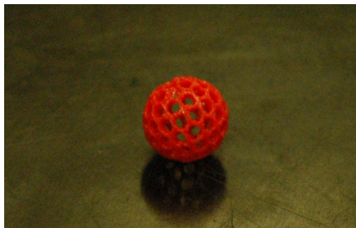
Figure 5.1: A porous sphere fabricated in a 3D printer of radius a = 8
