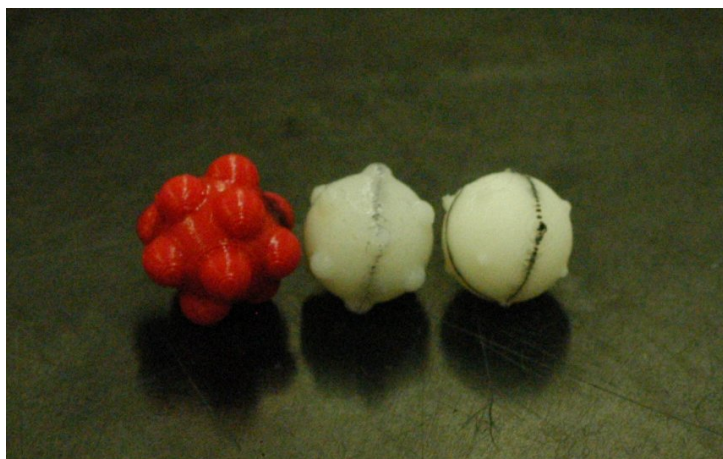
Figure 6.1: A picture of the three rough spheres used for this investigation. All the spheres have an inner radius of a_{min} = 6 mm and outer radius of a_{max} = 8, 7.5 and 7 mm respectively
