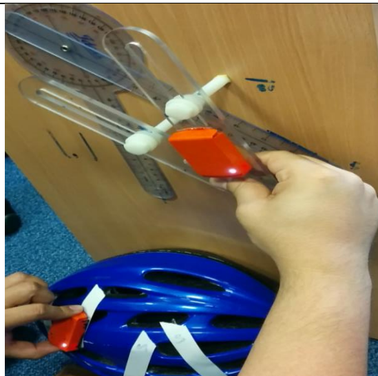
Figure 4.8. Scenario b), SL and humeral sensors placed on the wooden structure, simulating conditions similar to those found in clinical conditions. The scapula-sensor was placed in different orientations on a curved surface simulating the effect that the shoulder muscles can have on the shoulder.
