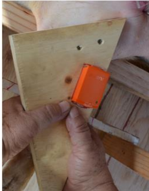
Figure 5.7. Traingular wooden base, used to fix the humerus and ulna of the pig leg and support the humeral sensor.
