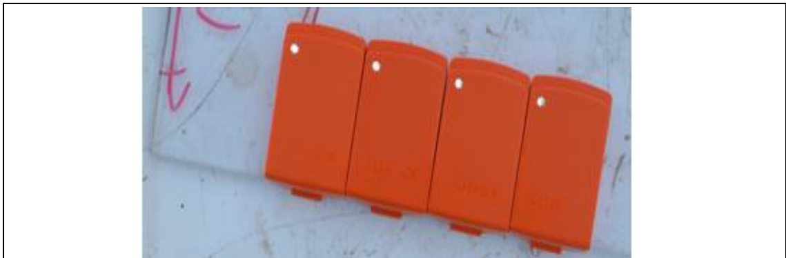
Figure 5.3. Four inertial measurement units (IMUs) were used for the porcine test.
