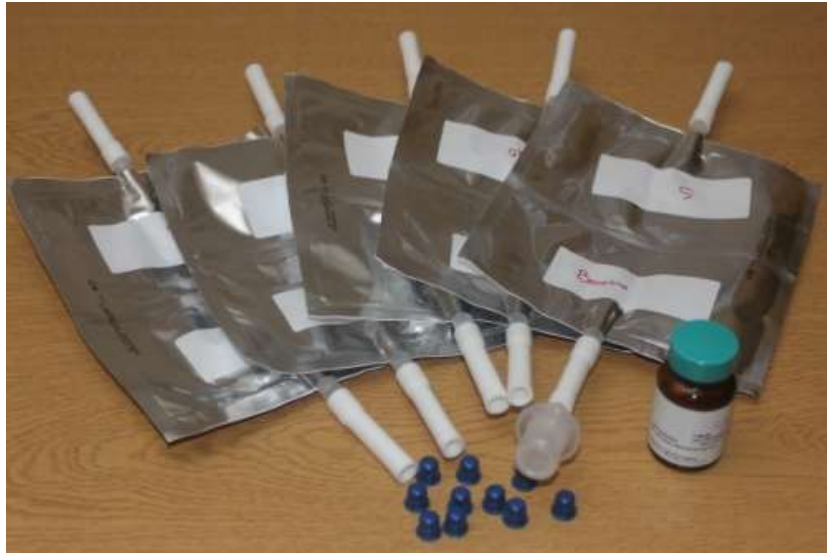
Figure 5.21: Sample bags, stoppers, mouth piece and sodium acetate
