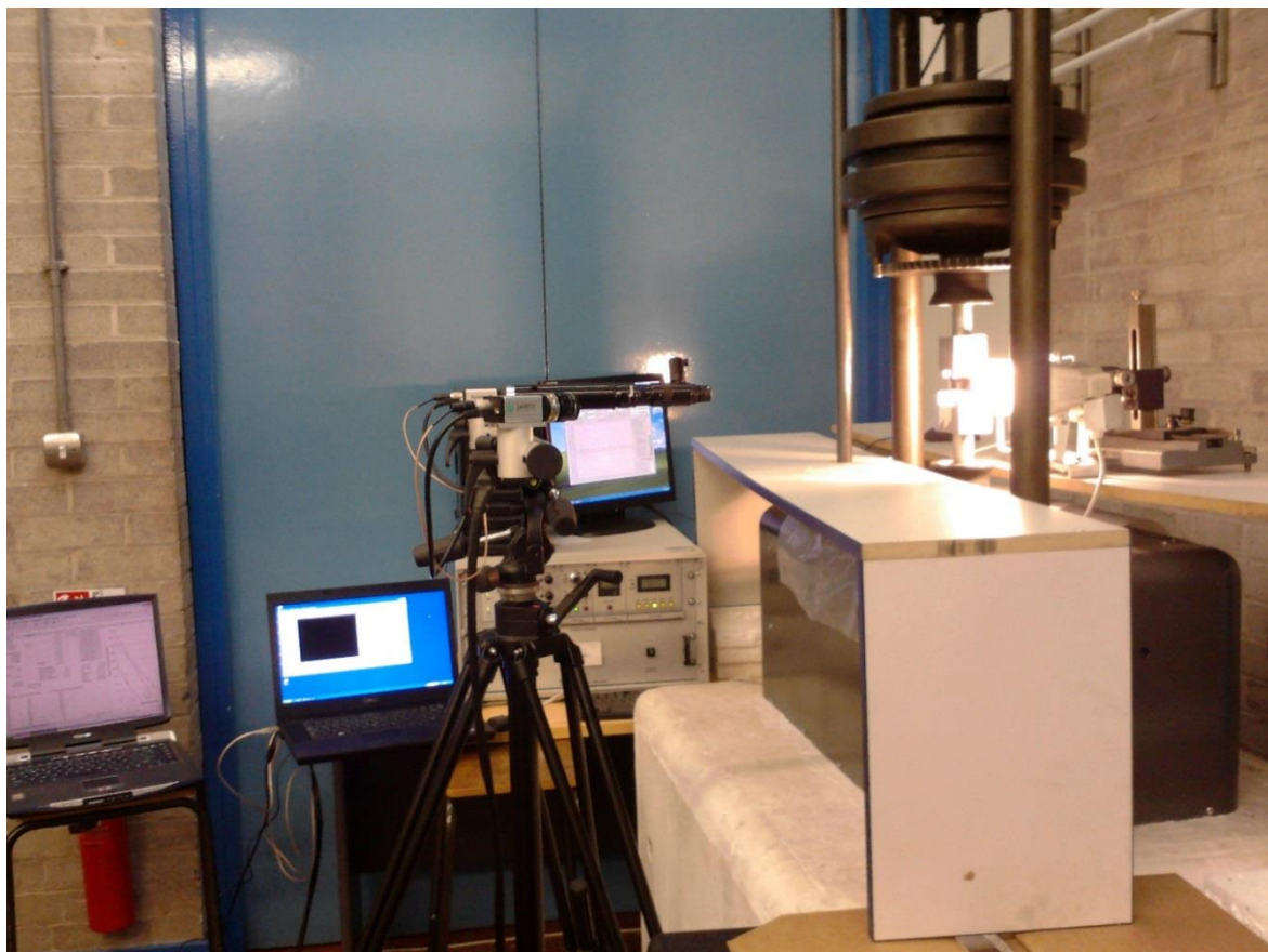
Figure 3.7: Set up of the Q-400 System ISTR A 4D. The figure shows the camera with the coupled telephoto lens (at the front), the data acquisition system, and the travelling microscope (to the right).
