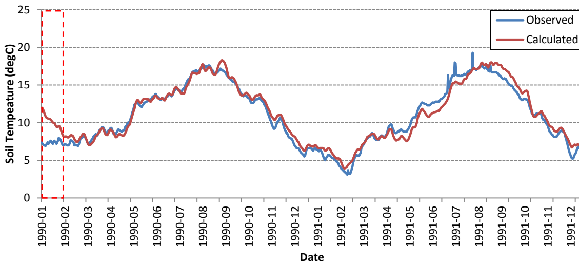
Fig. 2-24: Validation of the soil temperature model at 1 meter depth.
