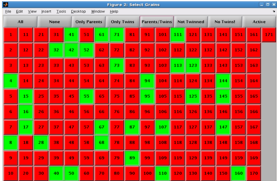
Figure 5.27: GUI for selecting/deselecting grains in the volume: pre-defined lists are available using the buttons on the top. In this example twinned grains and twins are selected.
