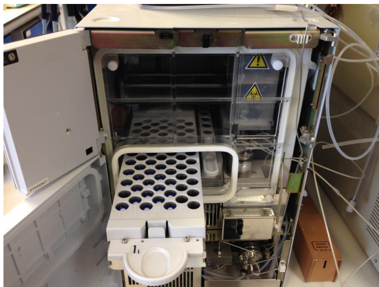
Figure 8: Auto sampler with sample rack exposed
