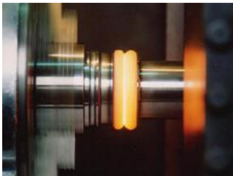
Figure 2.11 A photograph of rotational friction welding process [21].
