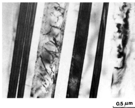
Figure 2.34 Deformation twins observed in a \text{Al}_3\text{Ti} specimen deformed at 25 °C [92].
