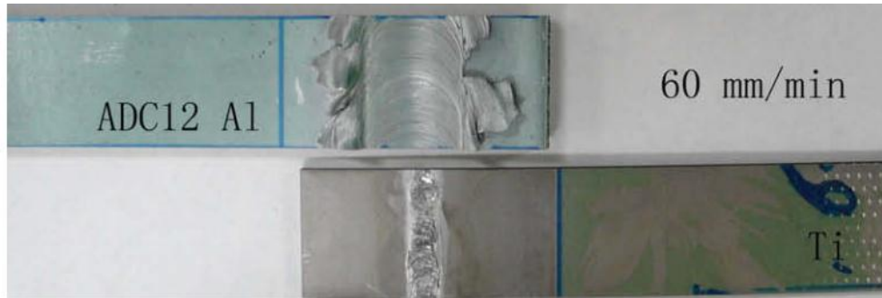
Figure 2.7 A typical fractured Al-Ti friction stir lap weld [12].
