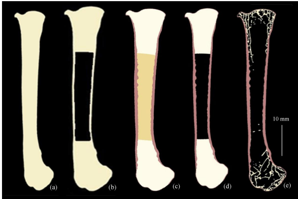
Figure 2 Two dimensional slices through the segmented image showing masks for (a) level 1 - a solid bone with one type of material; (b) level 2 - a solid bone with one type of material and a hollow cavity; (c) level 3 – a two phase bone with solid cancellous bone, solid cortical bone and a hollow cavity (shown in yellow); (d) level 3 – with the mask for the hollow cavity removed using a Boolean operation and (e) level 4 – with a full resolution mask for the cancellous bone including all the internal micro-structure.
