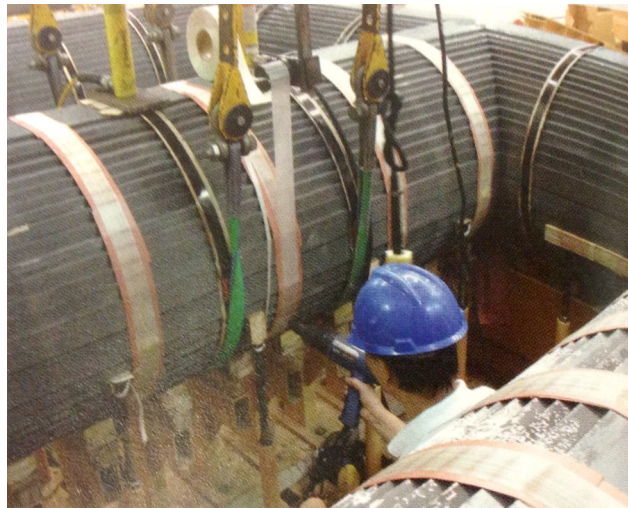
Fig. 3.7 Boltless core tightening with the glass fibre [3].
