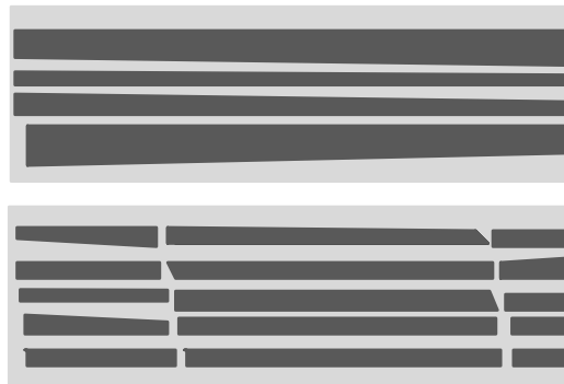
Fig. 6.4 Domain refinement of GO steel by the laser scribing.
