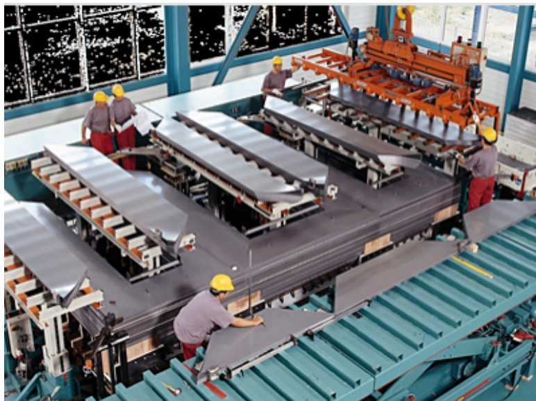
Fig. 3.6 Labour-intensive transformer core stacking [3].
