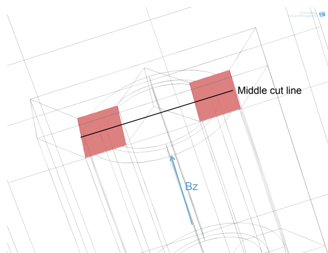
Fig. 7.27 The cut plane for the leakage flux under the bottom of the upper yoke.
