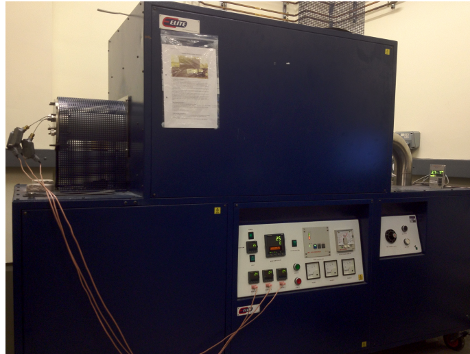
Fig. 4.2 Vacuum tube furnace used for the stress relief annealing.
