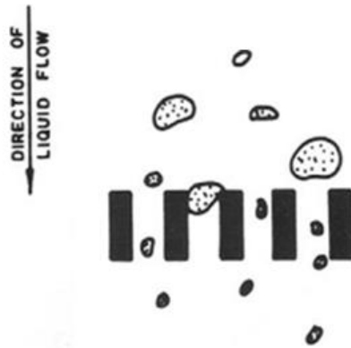
Figure 1.9 Filtration by surface straining [65]
