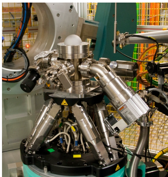
Figure 2.10: Picture showing the I07 beamline ‘baby’ chamber mounted on the hexapod.
