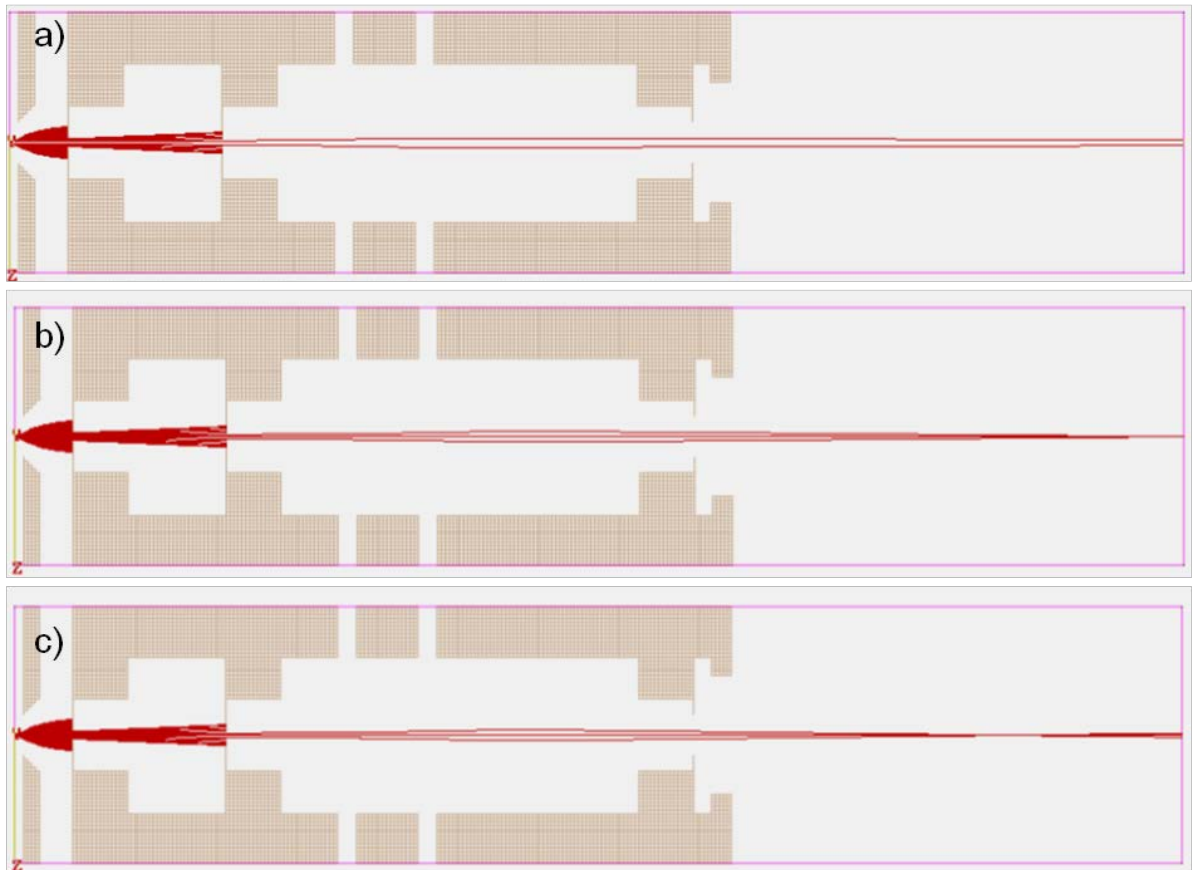
Figure 18 - a) Lens element held at 0 V b) Lens element held at 250 V c) Lens element held at 300 V
