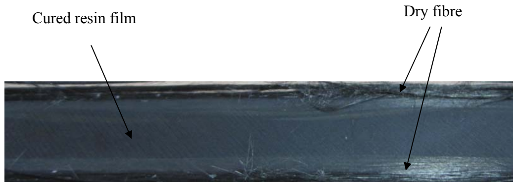
Figure B.2. Cross-sectional photograph of a cured composite manufactured using a thermoplastic-bound UD fabric. The photo highlights the cured resin film surrounded by dry fibre.
