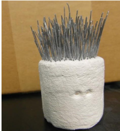
Figure 4.24 Fecralloy rods with alumina washcoat.
