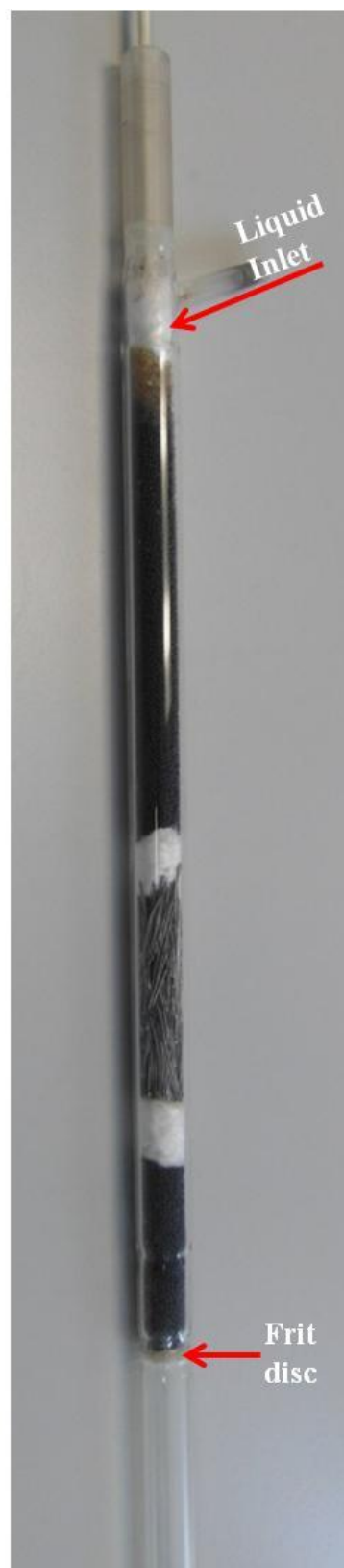
Figure 5.4 Glass reactor tube detailing gas and liquid inlets, central thermowell and glass fitted disc supporting catalyst.
