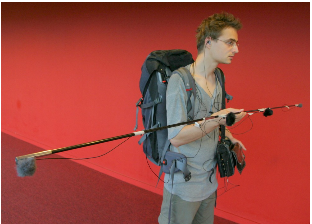
Figure 14: Photo of the complete recording set-up. Tentpoles had been used to attach the microphones.
