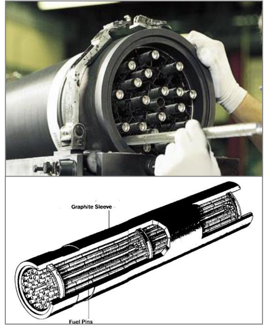
Figure 1.2. Photograph and diagram of the AGR fuel element's graphite sleeve inside which can be seen the stainless steel fuel pins.
