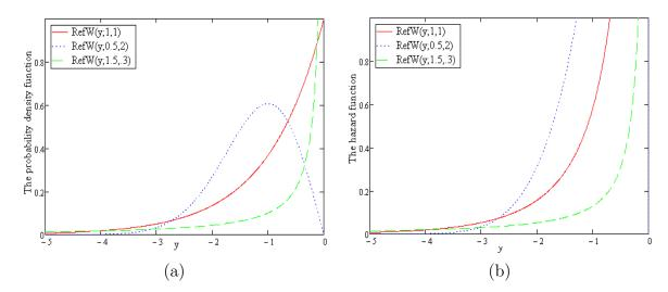
Figure 2.3: PDF and HF of the reflected Weibull distribution
