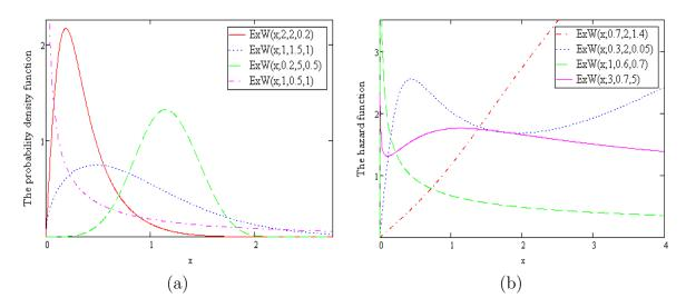
Figure 2.9: PDF and HF of the extended Weibull distribution
