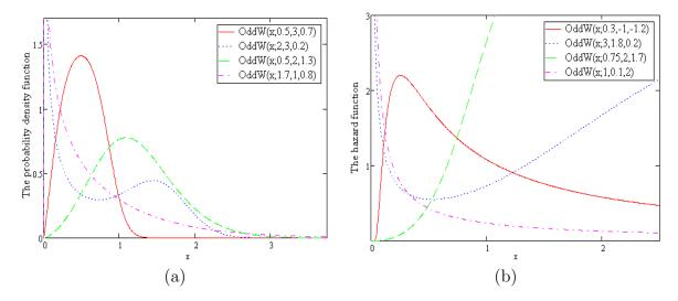
Figure 2.19: PDF and HF of the odd Weibull distribution
