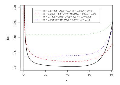
Figure 3.7: Hazard function of the NMW with a long useful life period.
