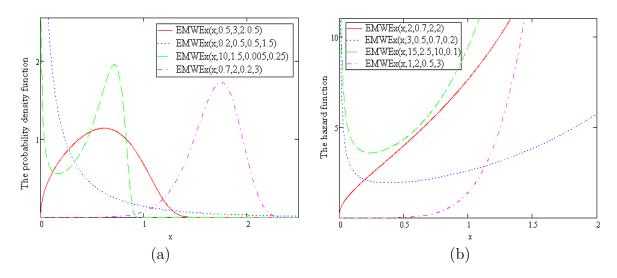
Figure 2.15: PDF and HF of the exponentiated modified Weibull extension
