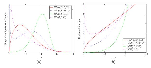
Figure 2.12: PDF and HF of the modified Weibull distribution
