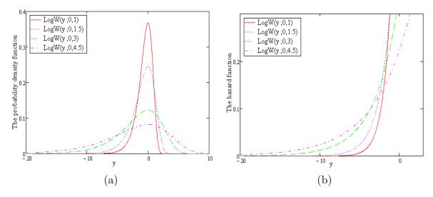
Figure 2.2: PDF and HF of the log-Weibull distribution
