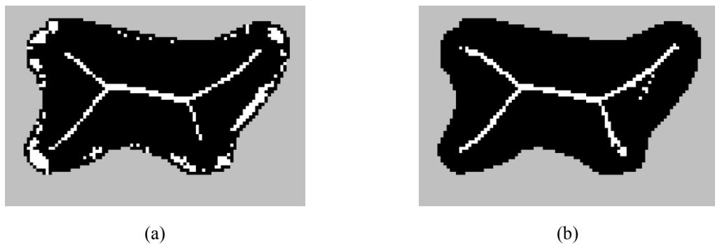
Figure 5.28. The skeletons of the same object extracted for: a) wave triggered from all the background pixels, and b) wave triggered only from the pixels on the border of the image.
