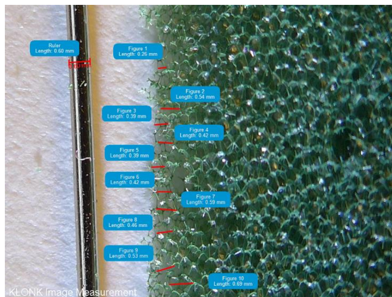
Figure 5-39. Measurement of porous size for the large porosity Styrofoam (Green). At the centre appears a needle. For the sampled porous, the average porous size is X_L=0.47 mm, \sigma_L=0.12 mm.
