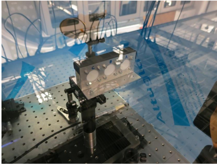
Figure 3-65. The triple cuvette mounted positioned inside the Perspex box.
