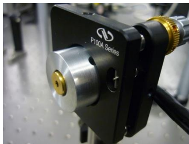
Figure A-1. Laser module in a mirror mount.
