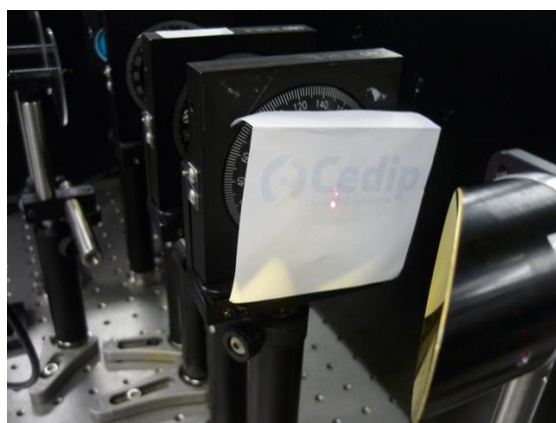
Figure A-17. Alignment of probe beam.
