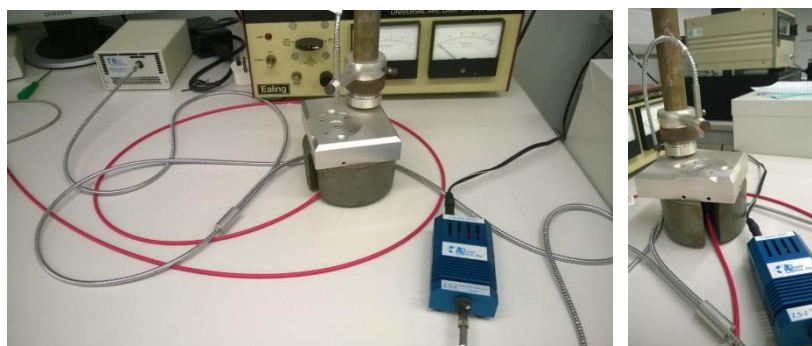
Figure 20 Absorbance equipment setup
