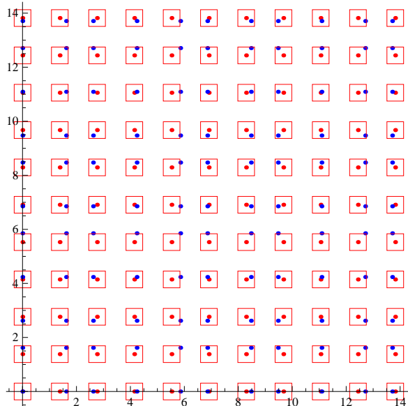
Figure 6.2: Square Fibonacci lattice vertices (blue), the PAS vertices (red) and the maximum range from the PAS vertices (red squares).
