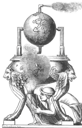
Figure 1- 1: Heron's steam rotor (Fransson, Hillon and Klein, 2000).
