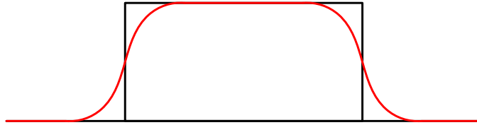
Figure 6.1: Hard edge magnet model; Real magnet field (red) and hard edge model (black).
