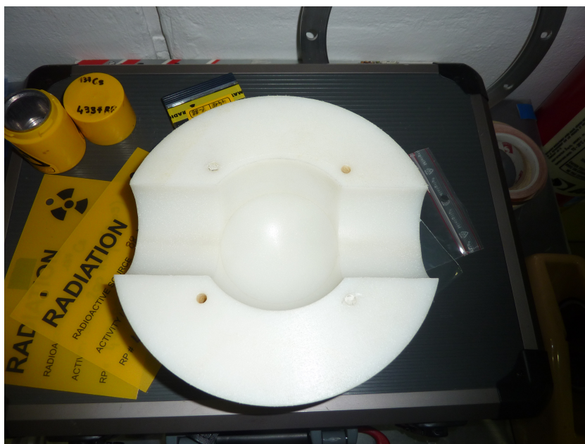
Figure 2.9: One hemisphere of the borated polyethylene neutron absorber used during the campaign to reduce the background from scattered neutrons.
