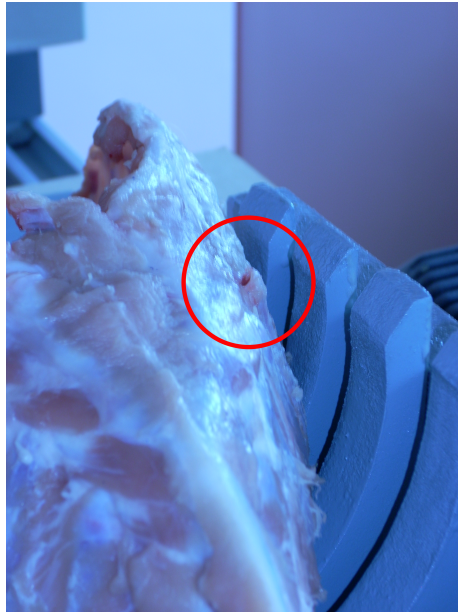
Figure 44. Photograph of external of Pig 2 thorax following abusive scenario mechanical test: red circle indicating costochondral failure to right rib 5
