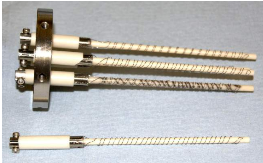
Figure 5.9: Photograph showing an assembled heater and all six heaters mounted onto the heater support.
