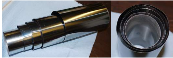
Figure 5.4: Photograph showing the five heat shields cut from thin molybdenum sheets and spot welded using a thin piece of tantalum strip. When mounted around the crucible, they are separated by thin-walled ceramic rods.
