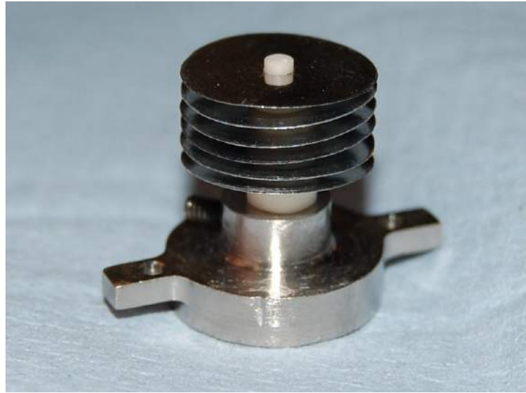
Figure 5.5: Photograph showing the "N-plate" holding a ceramic rod onto which six heat discs are mounted.
