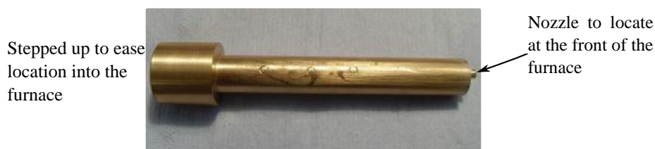
Figure 5.15: Photograph showing the custom-made alignment tool which substitutes the oven crucible in the process of aligning the oven to the interaction region.
