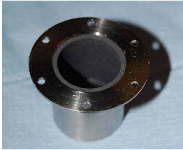
Figure 5.10: Photograph showing the graphite lining inside the skimmer cylinder. This ensured the skimmer remained re-usable by preferential sacrificing of the graphite.
