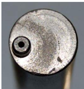
Figure 5.6: Photograph showing the nozzle at the front of the graphite crucible. The nozzle acts as emission hole from which the target vapour escapes the oven. As can be seen, it is offset from the centre to allow the maximum possible amount of sample to be loaded into the crucible.
