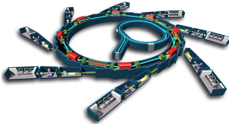
Figure 2-2-3. View of a synchrotron source which generates a high intensity of X-ray. Electrons are accelerated around a very large ring to nearly the speed of light. As the electrons are constantly accelerating, very high intensity radiation is emitted at a tangent to the curve of the ring. http:
