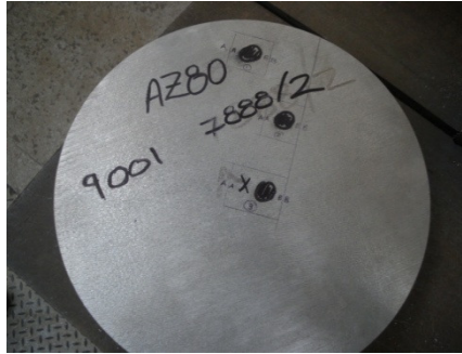
Figure 3-3 AZ80 billet slice marked for sample cutting.
