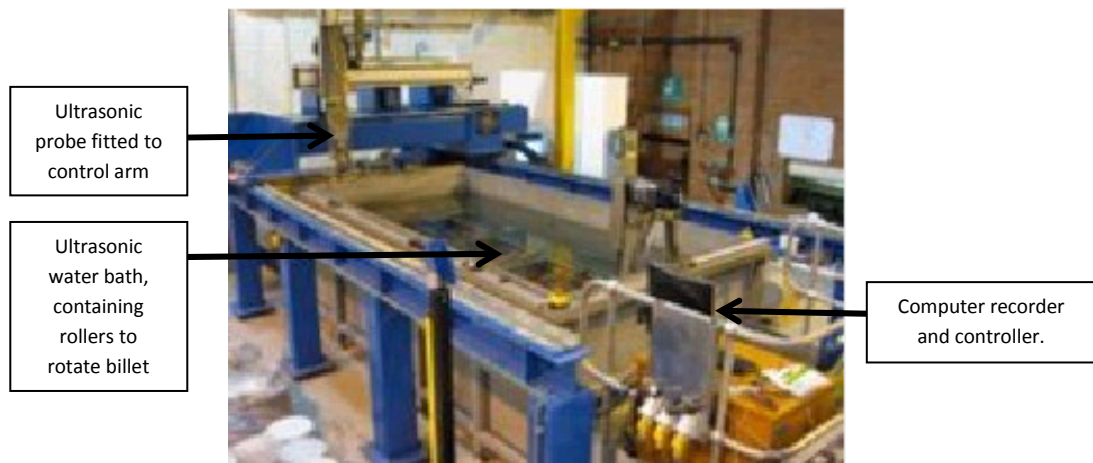
Figure 3-1 GE Inspection custom ultrasonic immersion tank.
