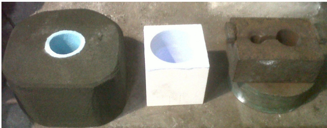
Figure 3-4 Photograph of moulds used for experimental castings; (left) sand, (middle) ceramic, (right) steel chill on copper block.
