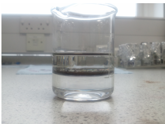
Figure 3.1: Lead sulfide thin film formed at the water-toluene interface.
