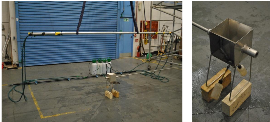
Figure 5-39 Calibration for the Spray System (Precipitation Rate Measurement)
