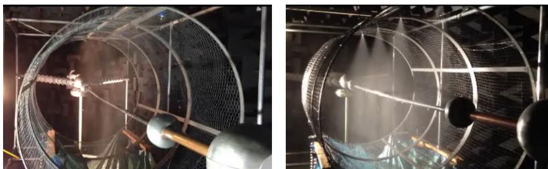
Figure 5-38 Light Spray Condition (left) Compared to Heavy Spray Condition (right)
