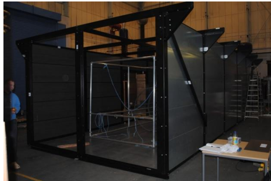
d). half-assembled anechoic chamber
