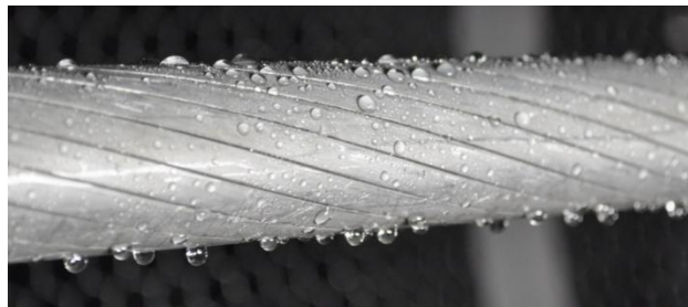
Figure 5-37 A Section of Conductor after Manual Spray Process
