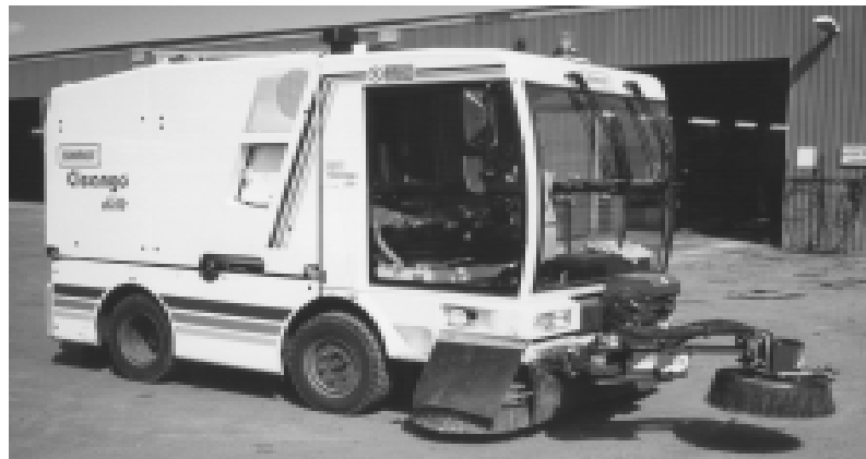
Figure 2 A mechanical brush street sweeper (German & Svensson, 2002)
