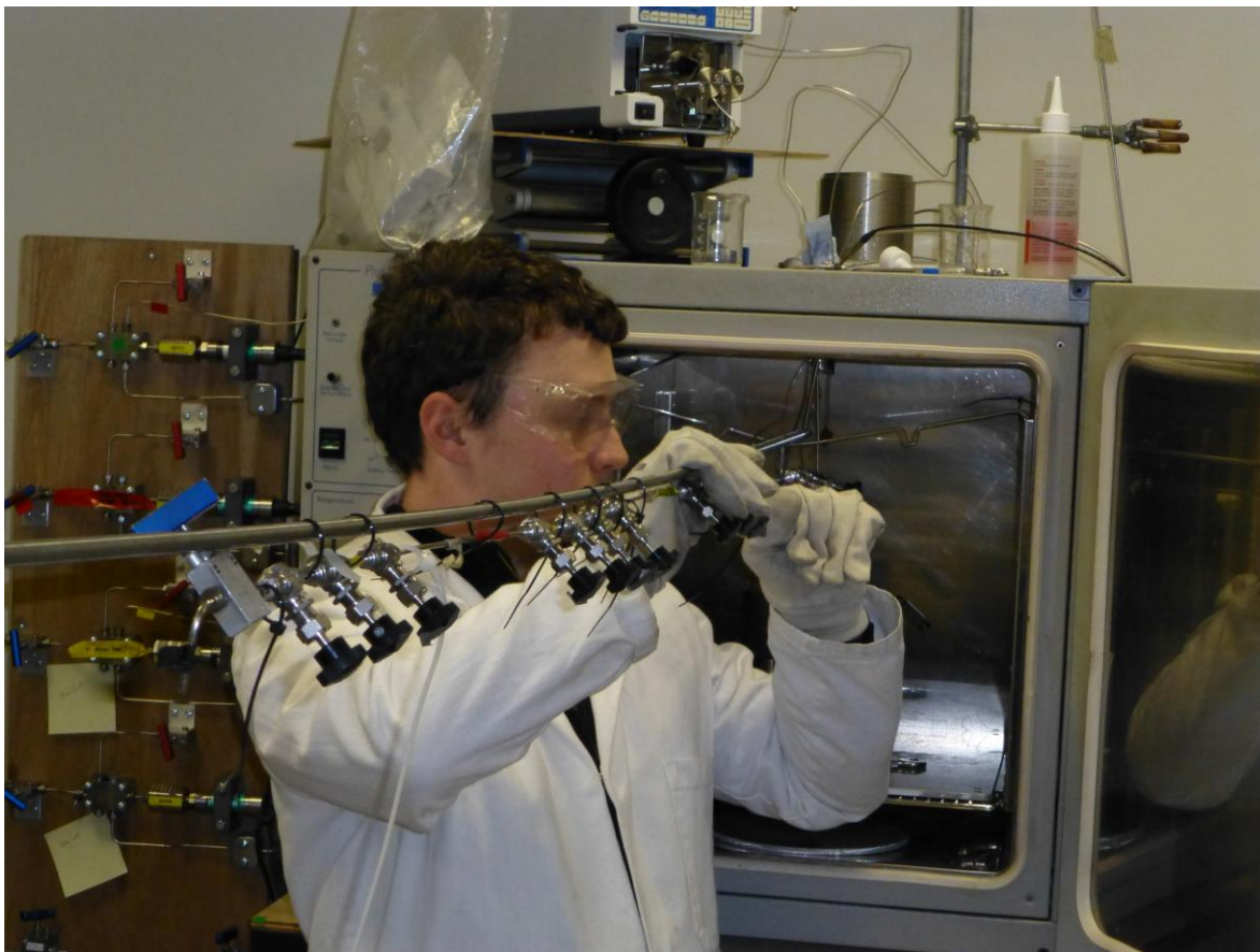
Fig. 2.8. Opening the sampler valves on samplers A1, A2 and A3 to sample the CO 2 phase.
