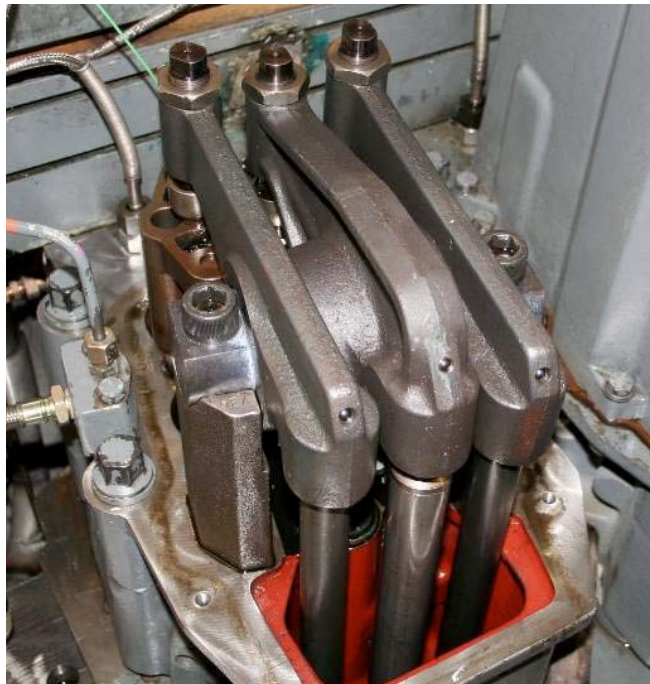
Figure 5.8: 6RK215 Cylinder One With Rocker Cover Removed
