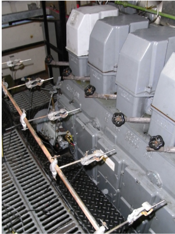
Figure 5.12: Microphones Installed on the Ruston 6RK215
