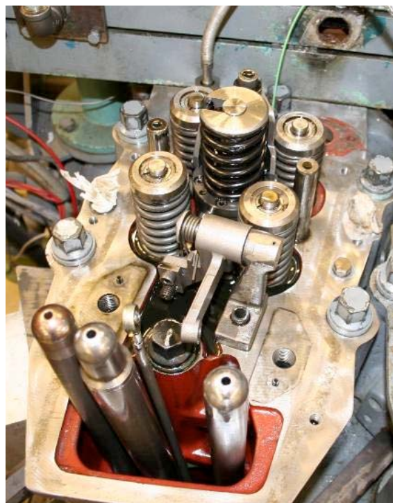
Figure 5.9: 6RK215 Cylinder One With Rocker Unit Removed
