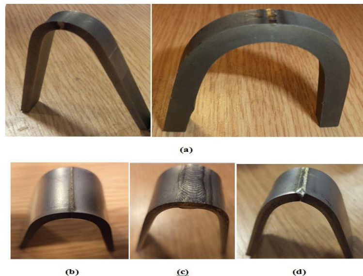
Figure 8-6 Bending test results for different weld samples
