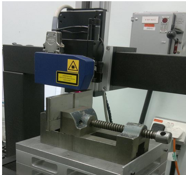
Figure 9-4 Nano laser scanner for relaxed surface scanning
