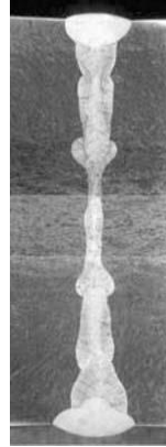
Figure 4-36 Narrow gap welding of 50 mm thickness stainless steel [16]
