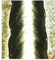
Figure 6-25 Optimum condition surface bead colour
