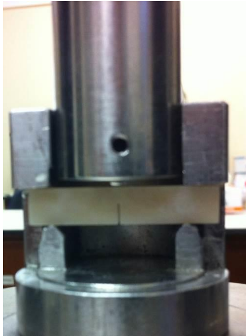
Figure 3.6: KIC specimen mounted on a cast metal jig
