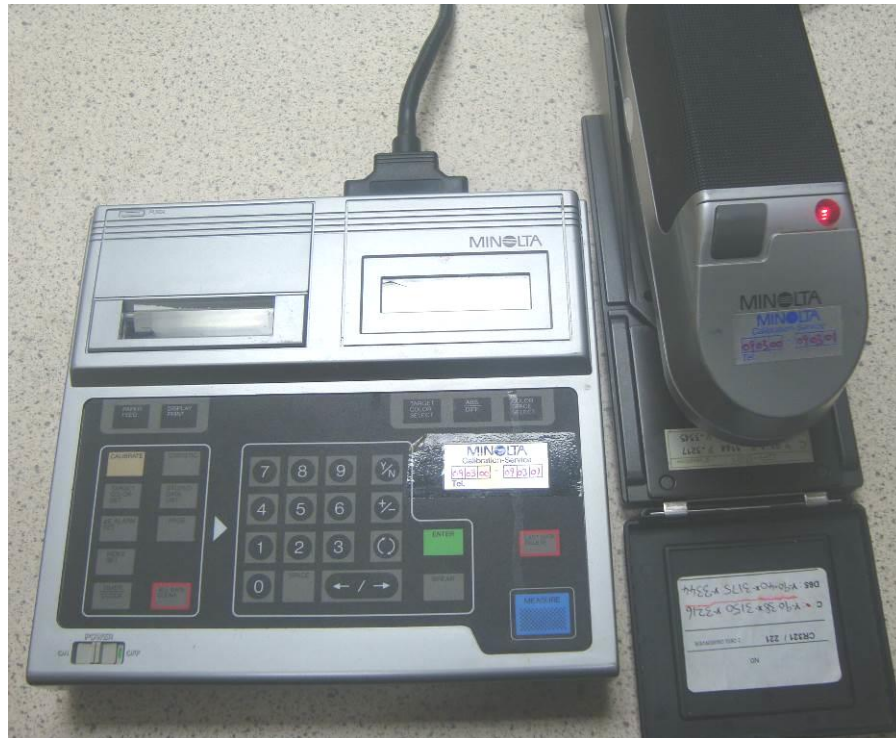
Figure 3.7: Chroma Meter instrument
