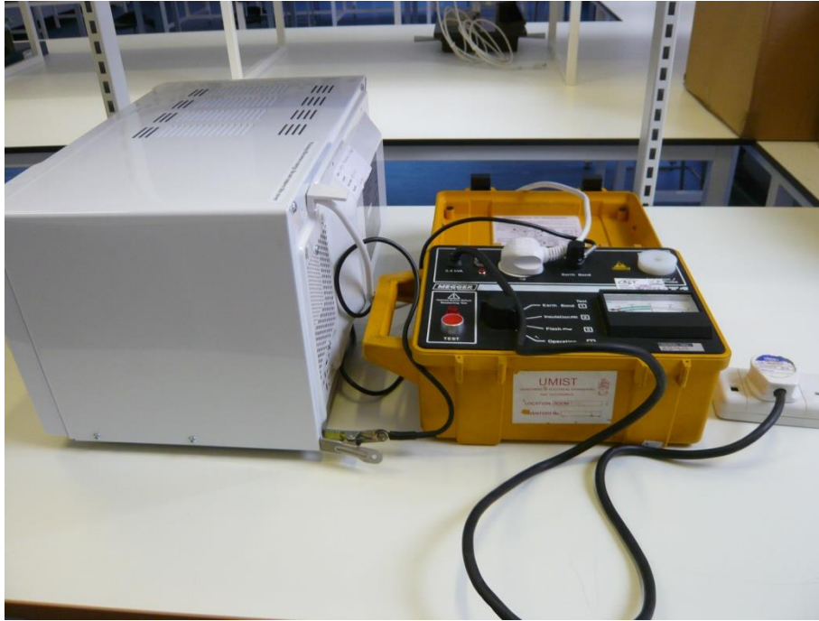
Figure 4.6: An illustration of the test arrangement for the PAT test at the University of Manchester
