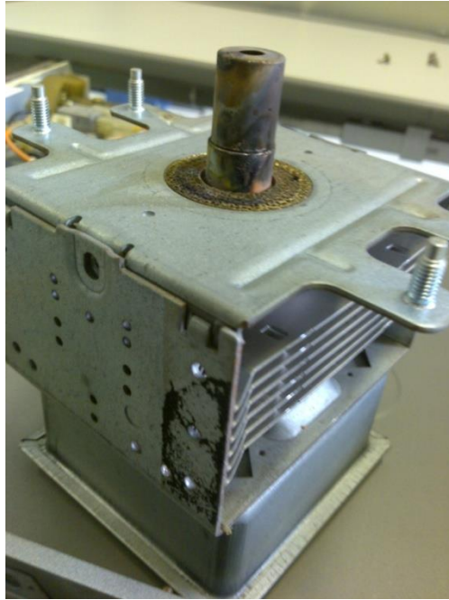
Figure 4.19: An arcing magnetron
