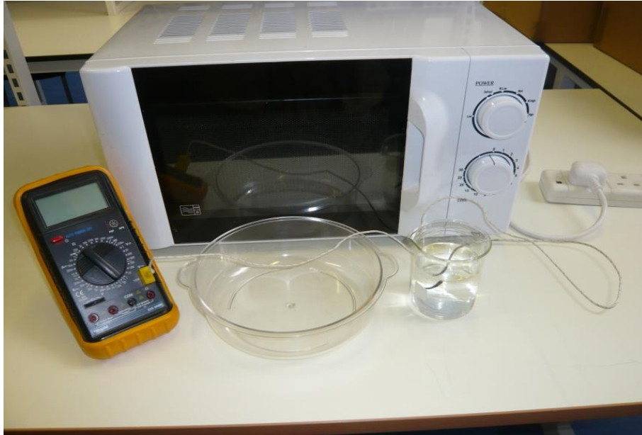
Figure 4.8: The equipment used to carry out the power test of the oven
