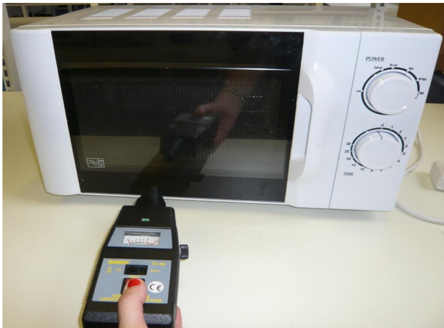
Figure 4.9: The microwave leakage test
