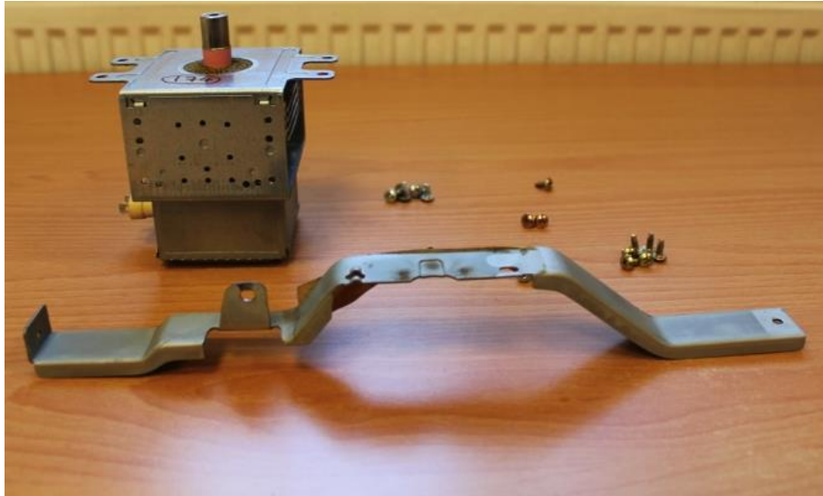
Figure 5.13: The disassembled magnetron from an oven and the screws used for its assembly
