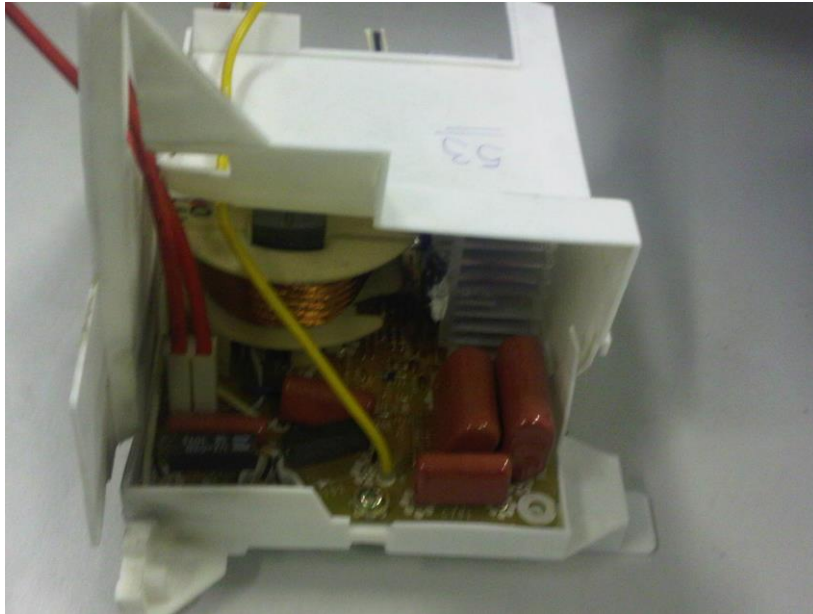
Figure 3.4: The inverter used within a microwave oven
