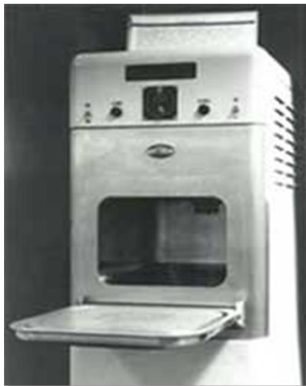
Figure 3.1: An early version of a microwave oven, Radarange developed, 1946 [128].
