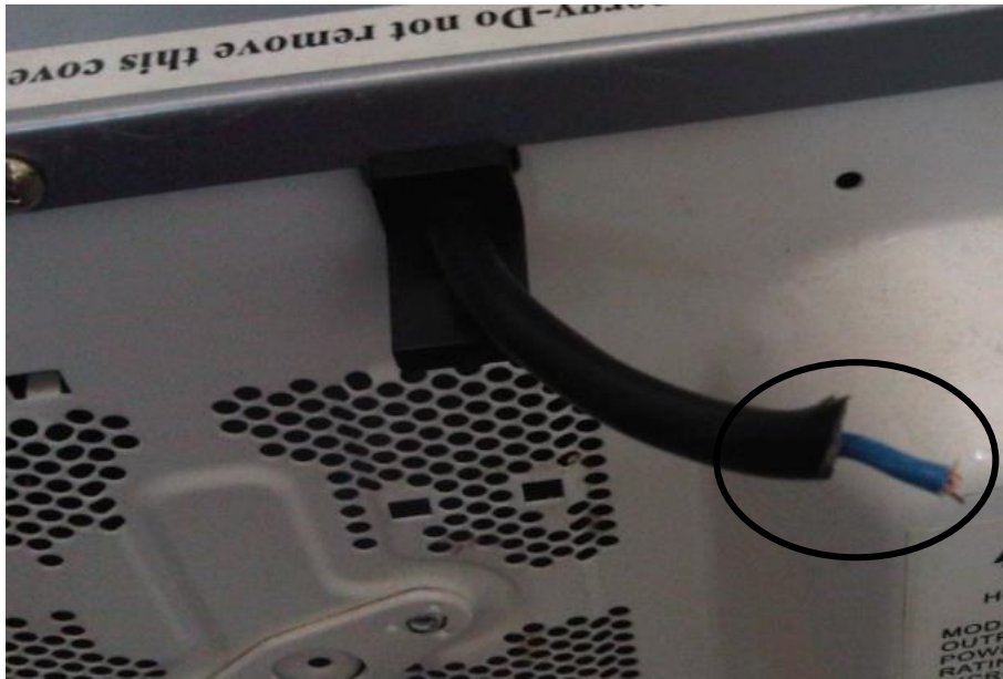
Figure 4.12: An example of damaged cord of a microwave oven
