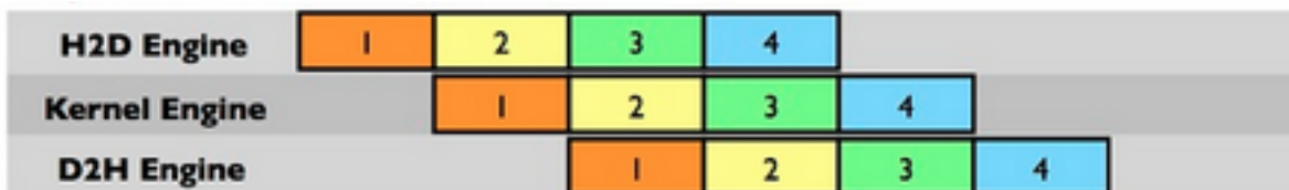
Figure 7.4: Asynchronous Memory Transfer [30]
