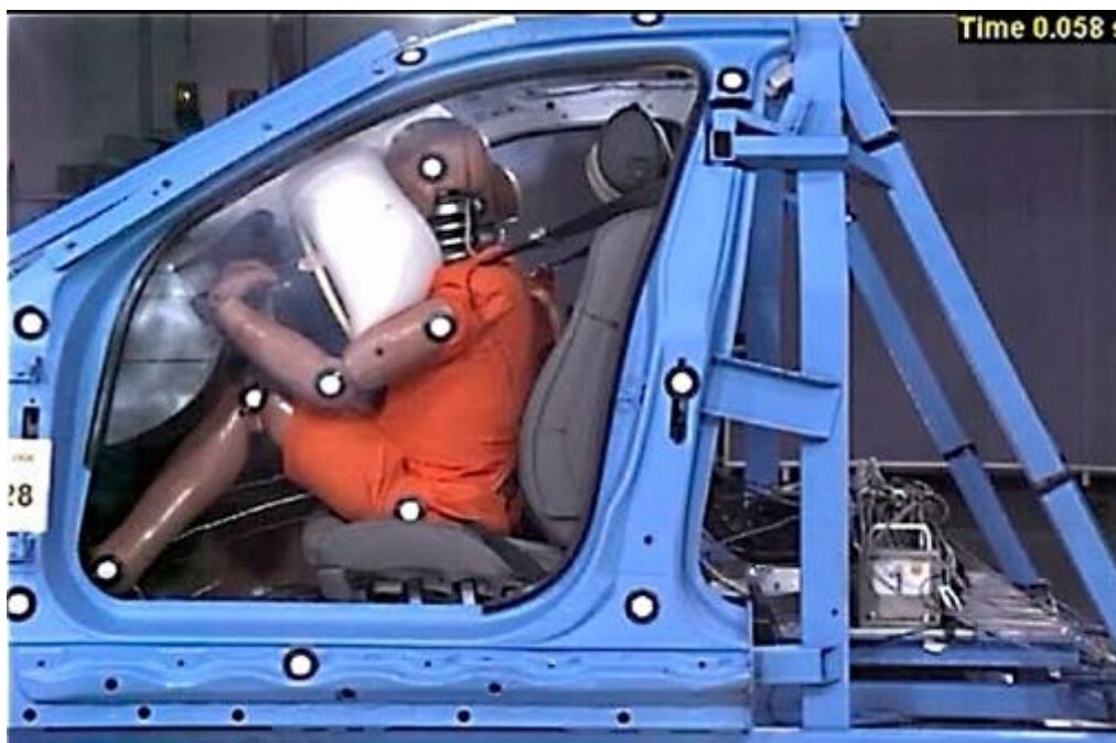
Fig 1: Airbag deployment during crash testing. (Source: Autoliv)
