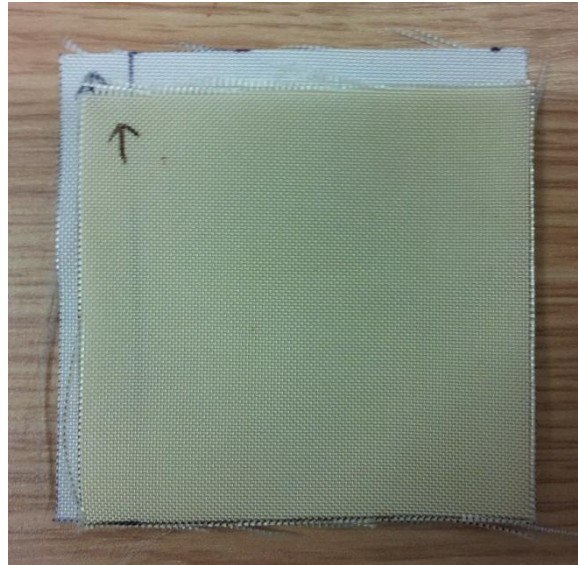
Fig 29 (b): Unheated and heated samples placed on top of each other with the arrow indicating warp direction.
