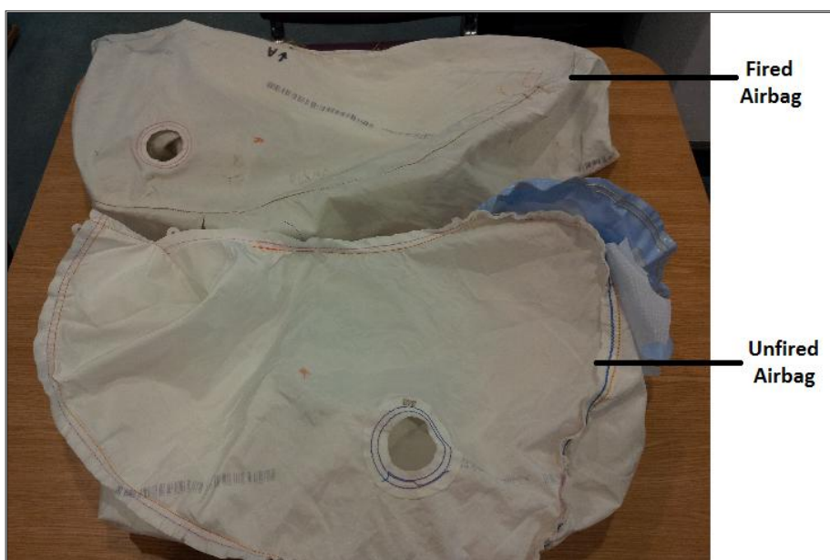
Fig 23: Right side panel of fired and unfired airbags
