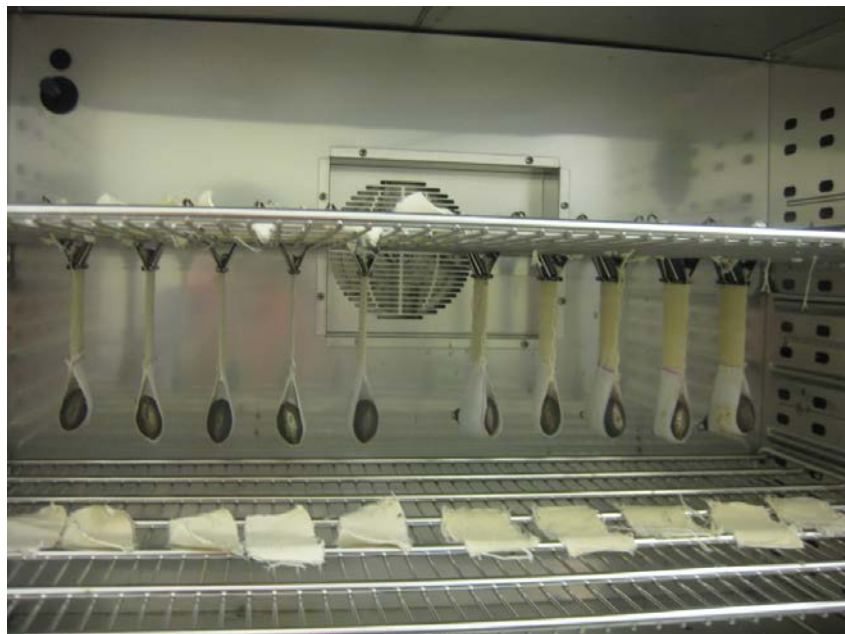
FIGURE 2.19 INTERIOR OF RH AGEING CHAMBER SHOWING BOTH HANGING AND STATIC SAMPLES
