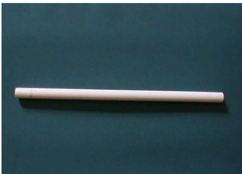
Figure 3.1: Virgin ceramic TiO 2 NF membrane with pore size of 1 nm.
